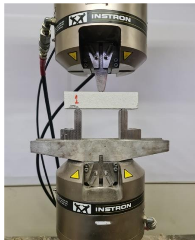
Figure 4: Testing of Flexural Strength
