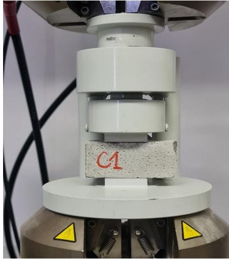
Figure 3: Compressive Strength Testing
